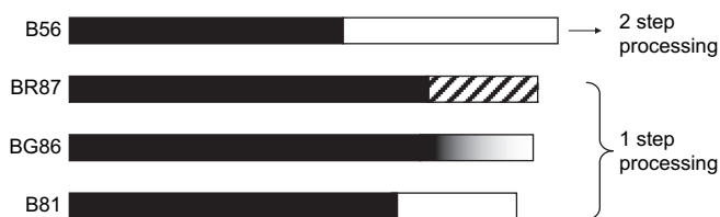
Fig. 1. Schematic illustration of styrene (S)/hydroxystyrene (HS) copolymers used as compatibilizers for PS/PCL melt blends. B56: a symmetric S/HS diblock copolymer consisting of one S block and one HS block, BR87: a diblock copolymer consisting of one S block and one short block of S/HS random copolymer, BG86: a diblock copolymer consisting of one S block and one short block of S/HS gradient copolymer, and B81: an asymmetric S/HS diblock copolymer consisting of one S block and one short HS block.
